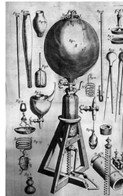
Some of the apparatus Boyle used to prove his law of gases
