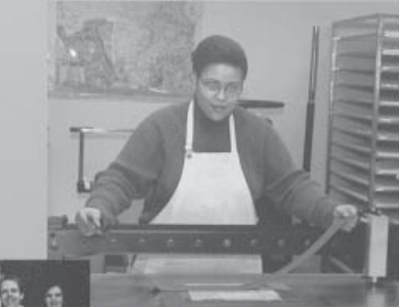
Conservation staff using the leaf caster to repair damaged pages.
